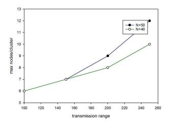
Fig. 5 Maximum number of nodes per cluster with different *R* for 50 and 40 nodes.
