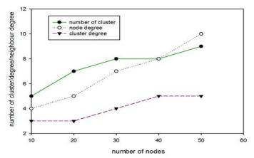
Fig. 4 Number of clusters, d (cluster degree) and  $\Delta$  (node degree) with different node number.
